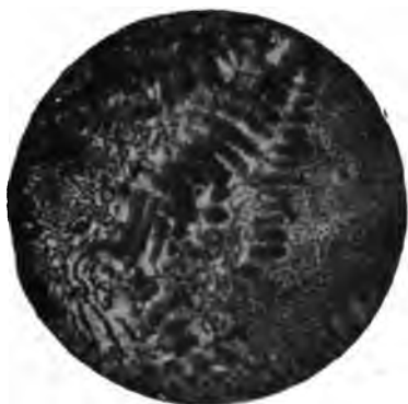
Fig. 17. Eutectiferous Copper-silver Alloy, Heat-tinted.
